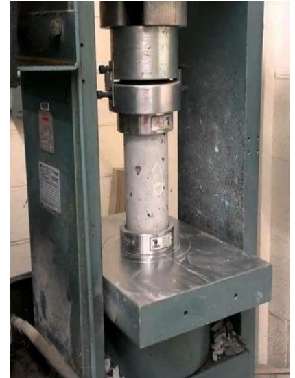
Fig. 5 - Compression Test by MTS Machine
