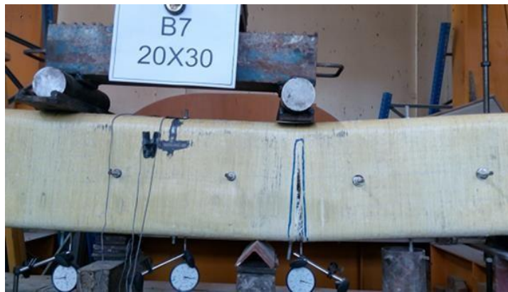
Fig. 8 - Failure Pattern of Specimens
